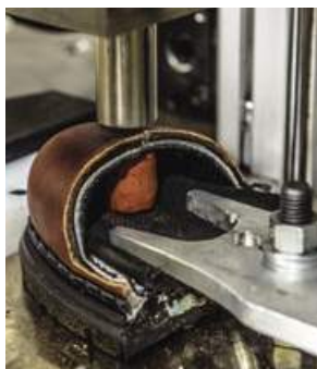
Left: The weight is dropped onto the protective toe cap area.
